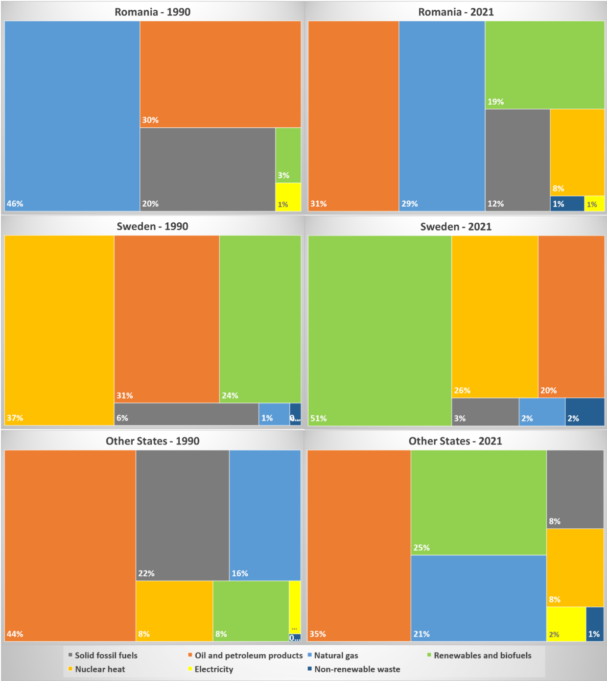
Figure 2.5 – Share of energy sources in gross inland energy consumption in the selected European states.
